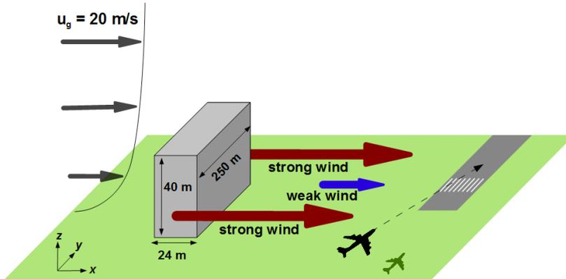
Figure 1: Schematic view of the simulated flight path through the wake of the building.
