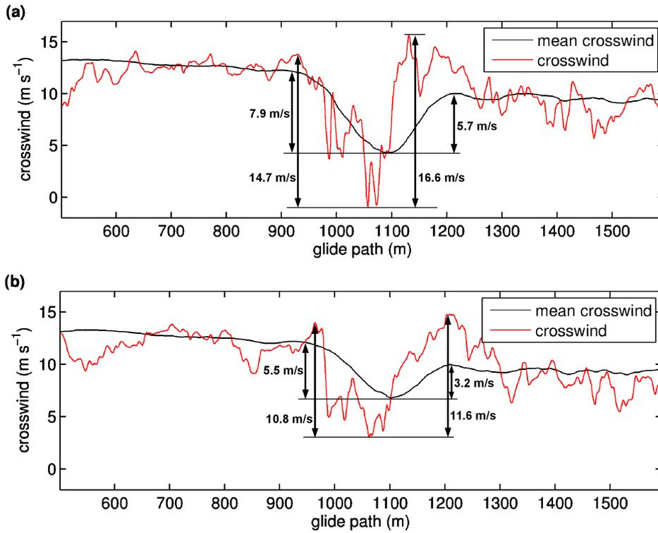
Figure 4: Virtual crosswind measurements along the glide path. The distances between the trailing edge of the obstacle and the glide path are 300 m (a) and 425 m (b).
