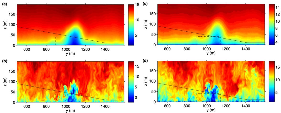
Figure 3: Vertical cross-sections of the mean (a and c) and instantaneous (b and d) crosswind in m/s downstream the obstacle (different color scales are used). The distance between the obstacle and the cross-sections is 300 m (a and b) and 430 m (c and d). The virtual flight paths are indicated by the black lines. For a better orientation the location of the building is shown by the dashed black lines.
