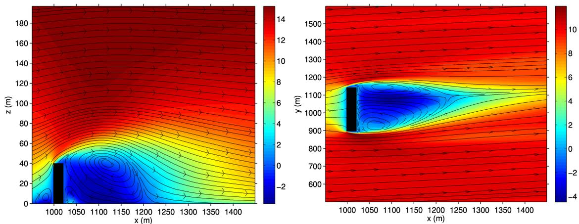
Figure 2: Mean flow around the building (black rectangle): Vertical cross-section in the middle of the building width at  $y = 1000$  m (left). Horizontal cross-section in the middle of the building height at  $z = 20$  m (right). The mean  $u$ -component (crosswind) in m/s is colored. Streamlines with arrows indicate the direction of the mean flow.
