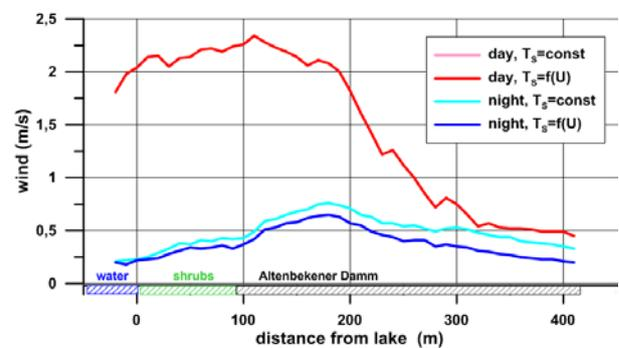
Figure 8: Simulated wind speed in 2m a.g. along the Altenbekener Damm for 14 hours (day) and 04 hours (night) for different water temperatures.
